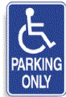
Each accessible parking space must be designated by a sign per [NH RSA 265: 73-a](#). Codes require that the sign display of the Universal Symbol of Accessibility and be mounted on a post or on a building wall so that the bottom of the sign is at least 60 inches above the surface of the parking space. Signs are to be located at the head of each accessible parking space. *Please do not use signs that have text with any form of the word "handicapped."*
